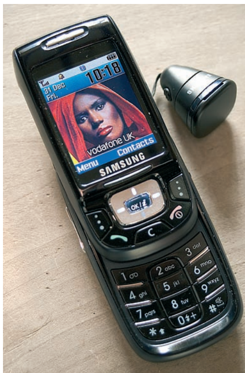
ABOVE: The Samsung D-500 cellphone (and hands-free loudspeaker) which has a built-in 1.3 megapixel (1524 x 1012 pixels) digital camera. The image of Grace Jones on the screen was uploaded to the phone from my picture library. The picture of the house (ABOVE RIGHT) was captured using this phone. Compare the 'quality' of this with the one in last month's issue using the Phase One P25. The picture of the guard on the preceding page was captured with a DCS420 with only a slightly higher number of pixels than the camera in this phone. BELOW: The forthcoming Kodak Easyshare-One with 3-inch screen features wireless connectivity using a special card. The camera was awarded CNET's 'Next Big Thing' and G4techTV's 'Best of CES' at the recent Consumer Electronics Show. Products such as this are what Kodak is pinning its hopes for the future on.
